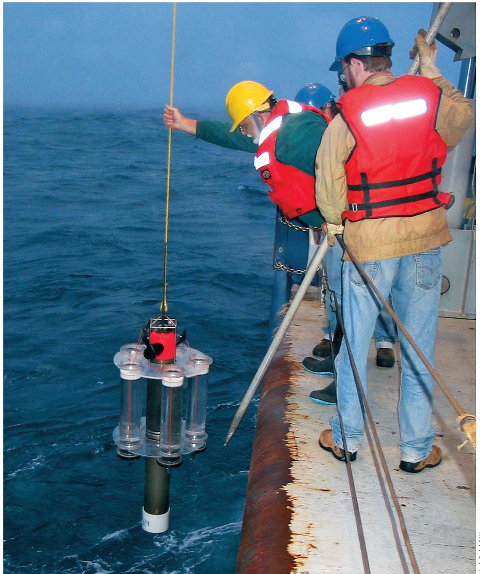
▲ WHOI biogeochemist Ken Buesseler (blue hat) and engineer Jim Valdes (yellow hat) deploy a Neutrally Buoyant Sediment Trap for a three-day mission in the depths of the North Pacific Ocean in 2005. The instrument collects "marine snow," the falling particles of dead phytoplankton and zooplankton feces that sink from sunlit waters into the ocean's "twilight zone."
