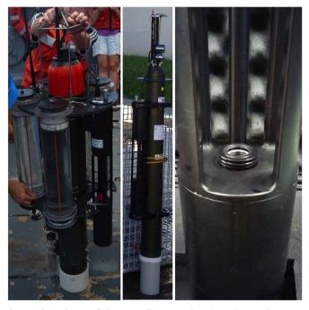
**Fig. 1.** Left panel: Neutrally-buoyant sediment trap (NBST) carrying 4 sediment trap tubes and an integrated C-Rover transmissometer (WETLabs C-Rover 6b). Center panel: Navis BGCi profiling float (Seabird Scientific) also carrying a C-Rover transmissometer (WETLabs C-Rover 2 K, identical in size and optical specifications to the C-Rover 6b). Right panel: Close-up photograph of the lower optical window of the C-Rover 2 K.
