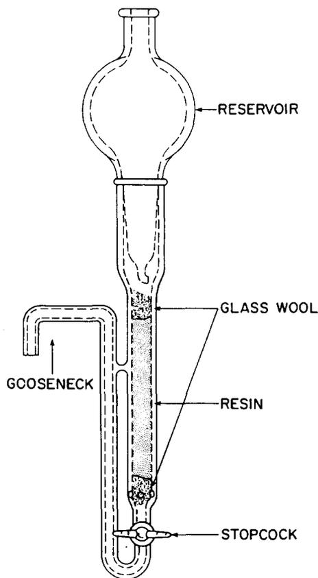
Fig. 1(a). 'Goose-neck' ion exchange column.
