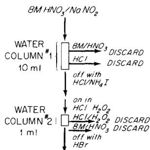
Fig. 2(b). Summary of ion exchange procedures for sea water, pore water, sediment trap and coral samples.
