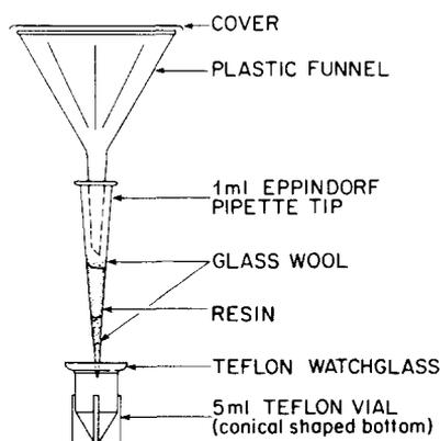
Fig. 1(b). 1 ml final ion exchange column.
