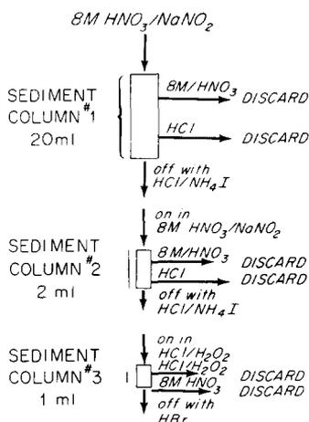
Fig. 2(a). Summary of ion exchange procedures for marine sediment samples.
