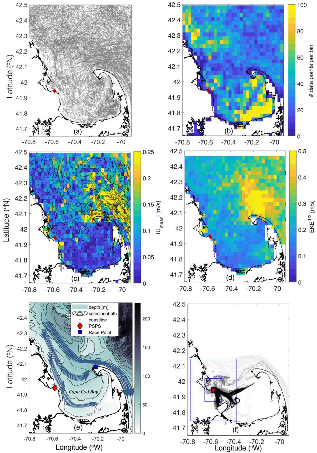
**Fig. 1.** For the drifter dataset used, spaghetti diagram showing trajectories of all available drifters (417 in total) deployed between 1989 and 2019 (a), number of data points per bin (b), mean velocity (c), eddy kinetic energy (d), schematic diagram showing the geometry of the flow in and around the Cape Cod Bay (e), and simulated trajectories advected by the mean field (f). In (f), black/dark grey/light grey trajectories start within the small/intermediate/large release boxes (blue
